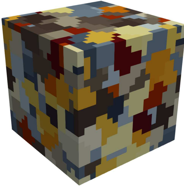
Figure 1. The polycrystal representative volume element containing 200 grains.
